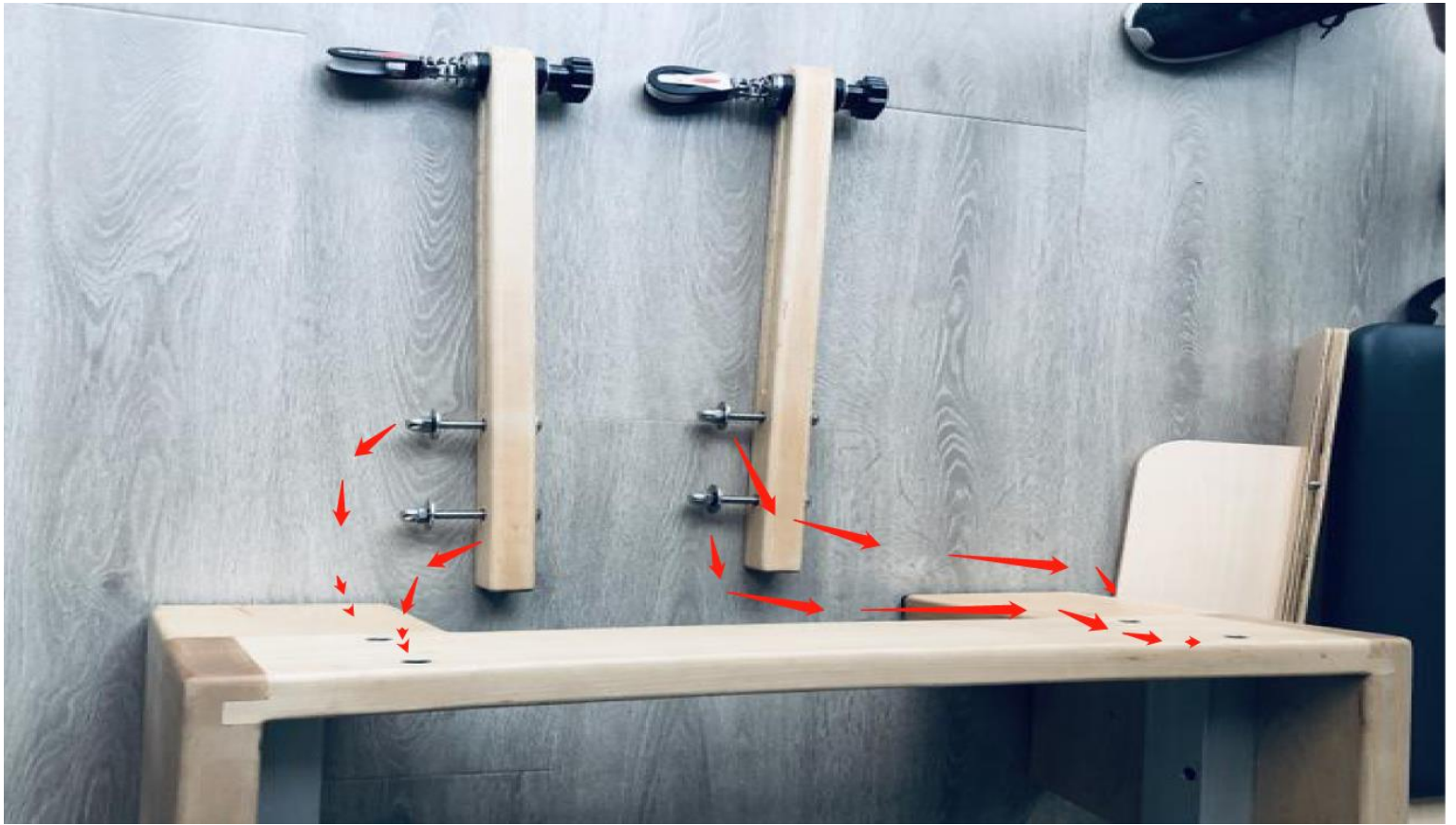
1.24: 拉绳杆组装 (参考普通核心床拉绳杆安装即可)。Assembly of rope pulling rod (refer to the installation of rope pulling rod of ordinary core bed).
