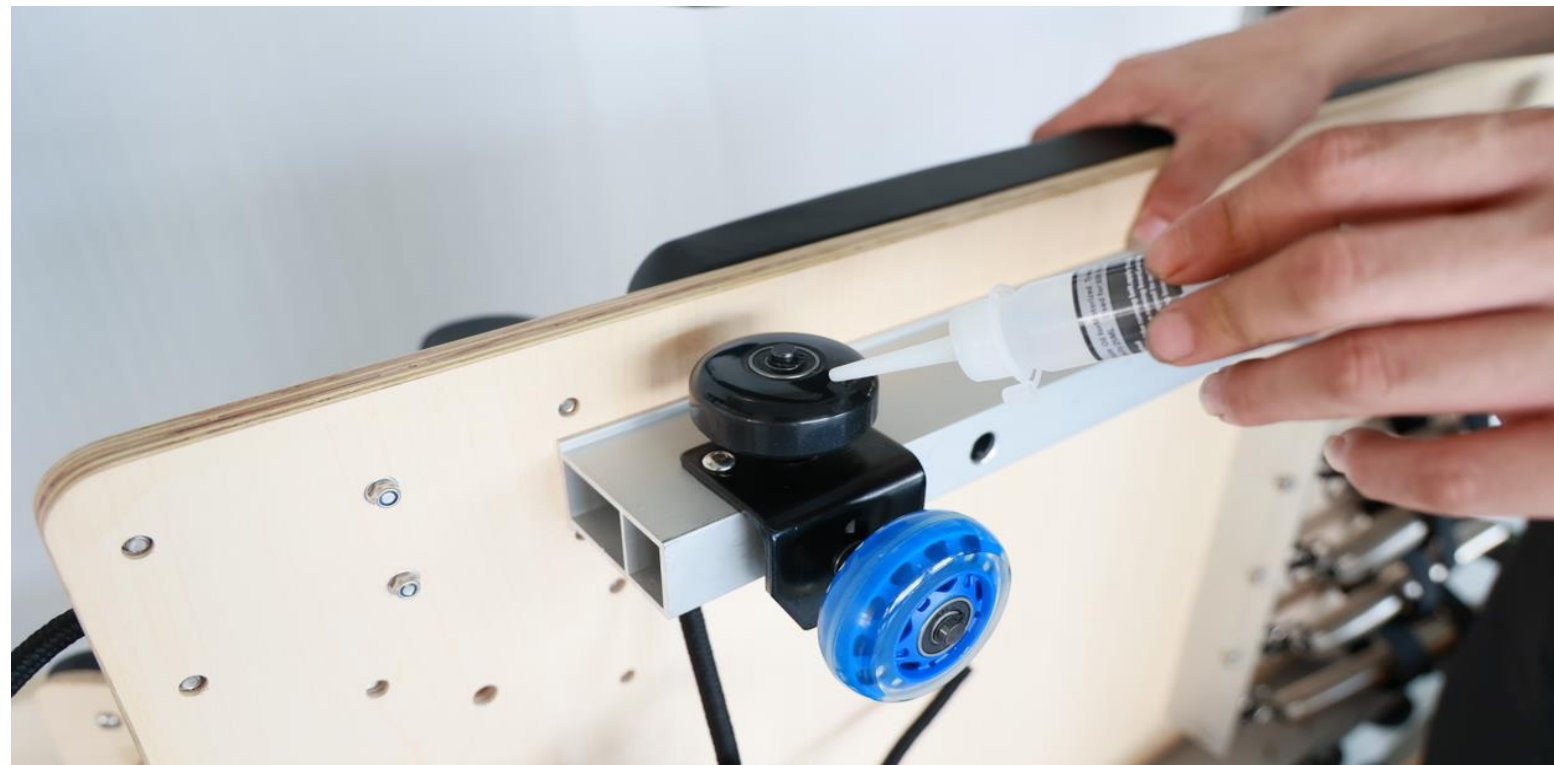
Silicone oil is added to rope pulling rod pulley.
