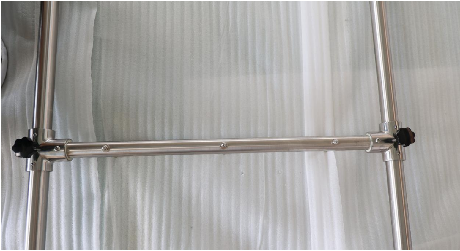
1.13-4: Installation of overhead jacking rod adapter.
